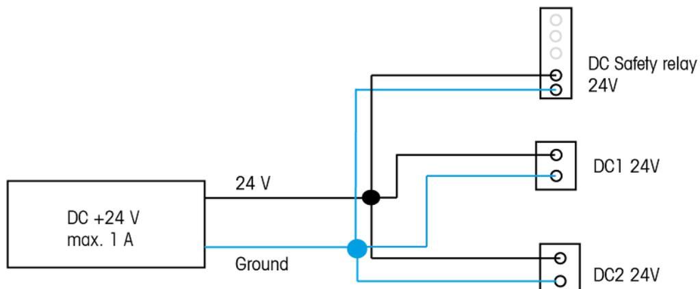
Contact your METTLER TOLEDO service to connect the electromagnetic valves to the safety relay of the RC1mx.
