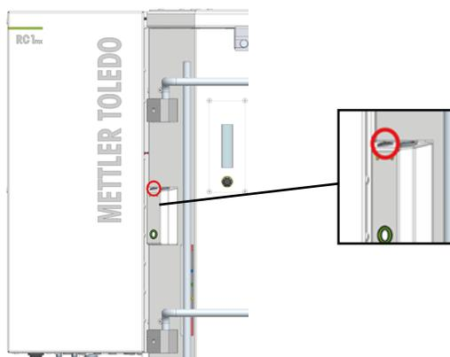
7 The Tr sensor connection is on the side of the instrument (see red marking).
